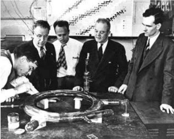
Scientists around the vacuum chamber of a 1947 General Electric synchrotron (photo courtesy of NSLS, Brookhaven).
